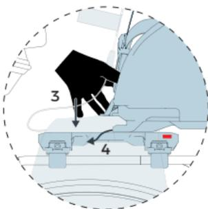
3. Press down the leg parts while sliding forward
