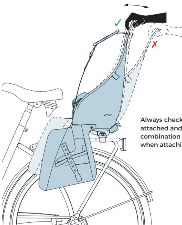
Always check to see if you properly attached and locked the cable with combination lock around the frame when attaching the bike seat.
