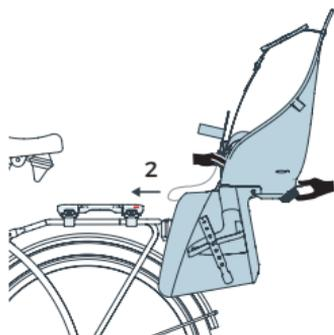
2. Slide the bicycle seat in a horizontal position over the bracket
